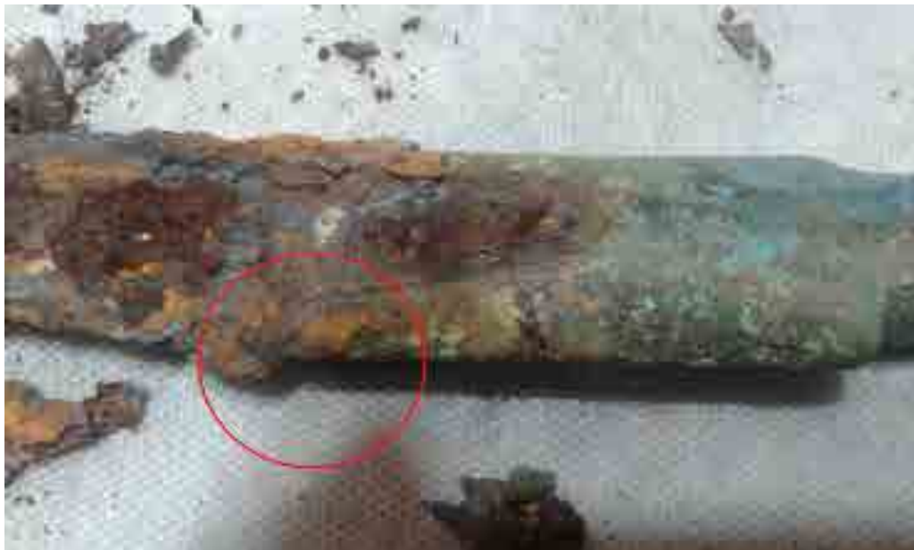
Fig. 13: Cathodic protection at the junction of the bronze handle to the iron blade (Original images: Soraya Mohammadi).
