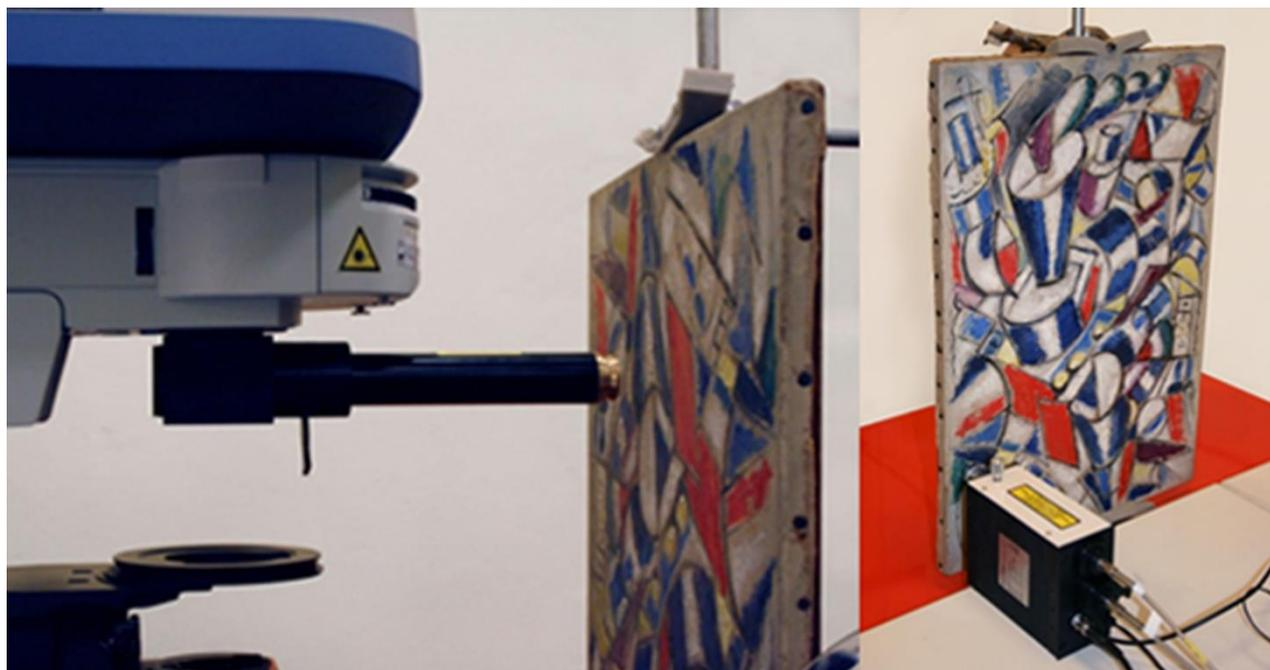
**Fig 3.** Device including 45° inclined mirror and tube and fibre optic configuration
